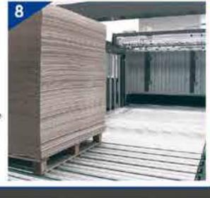
Automatic management of the pallets recovery from the loading area. to the unloading area. Original solution, patented by Elitron
