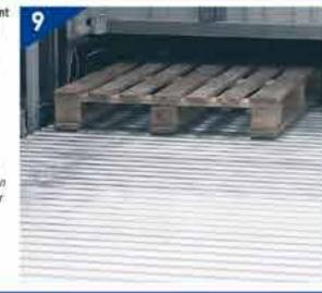
The material handling can be equipped with roller conveyors or Acetal mats, for the unloading functionality and even partial handling, up to the single sheet
