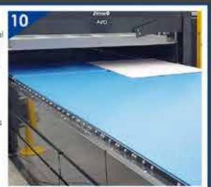
The system handles automatically the sheets pallets just processed. onto buffer areas, to be subsequently processed or collected
